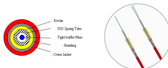
Figure 5.1.1 Structural Schematic of Temperature-Sensing Optical Cable
