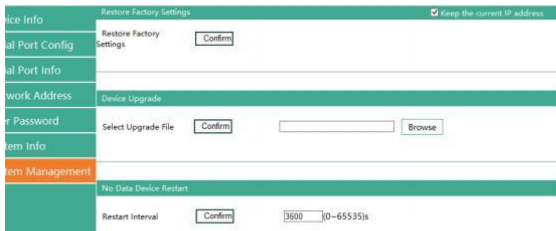
Figure 31 System Management Interface
