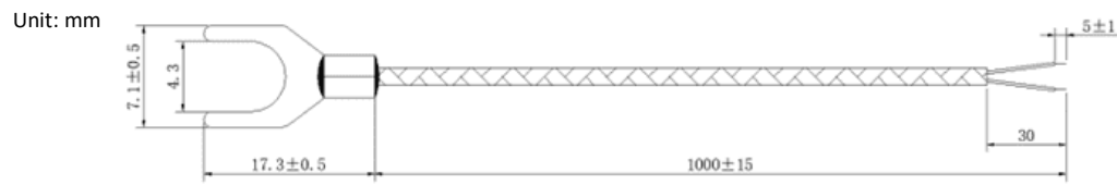
Figure 2-23 NTC-Y4 Dimensions
