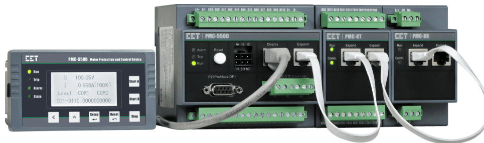
Figure 2-28 Connections with other modules
