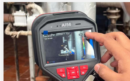
Gas Leakage Detection
