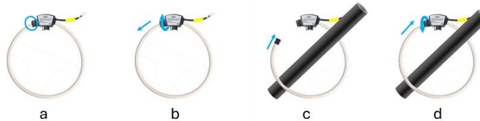
Figure 2-21 Rogowski Coil Installation Steps
